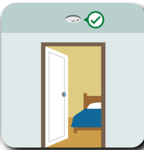
OUTSIDE OF SLEEPING AREAS, LIKE IN A HALLWAY
