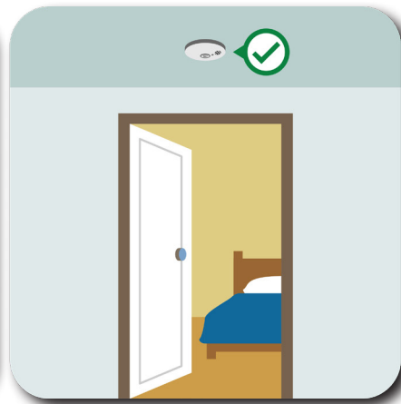
OUTSIDE OF SLEEPING AREAS, LIKE IN A HALLWAY
