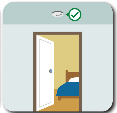
OUTSIDE OF SLEEPING AREAS, LIKE IN A HALLWAY
